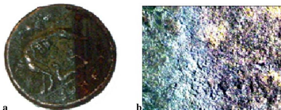
**FIGURE 2** a Laser cleaned Roman coin with both Q-switched  $2\omega$ -Nd : YAG laser (right side) and a TEA  $\text{CO}_2$  laser (left side) b Microscopic (40x) photo of the surface morphology
